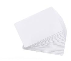
The MIFARE Classic 1K card from NXP operates at 13.56 MHz wireless frequency, according to the ISO 14443A standard, and contains 1K bytes of read/write memory that can be used for multiple applications. This version of the MIFARE Classic 1K Card has a unique 7 byte (56 bit) chip serial number/ID, instead of the older 4 byte (32 bit) variety.
